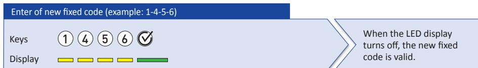
If you cancel the enter process of a new fixed code with the cancel button or if you enter an incorrect code (invalid code length), the code 1-2-3 will automatically be valid. In this case the LED display flashes red ten times.
