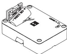
Insert the battery first with the minus pole as shown above. The battery is placed on the battery removal tape so that the tape tip protrudes.
