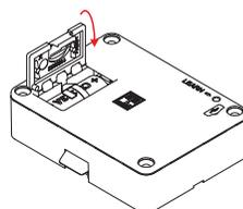
Close the battery compartment with the tape inserted.
