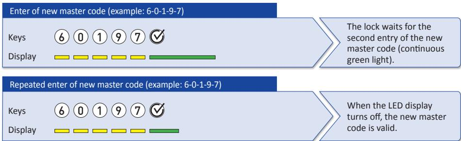
If the new master code has been entered correctly twice, there is a long green flashing in the LED display. The new master code is valid. In all other cases, the LED display flashes red ten times. The new master code was not accepted. The previous master code is still valid.
