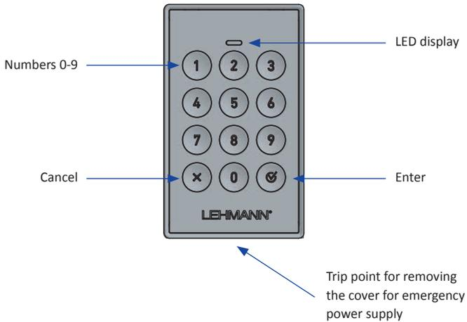
You can cancel any operation at any time by pressing the cancel button (X). When the cancel button is pressed, there is one short red flashing. Any input already made is deleted.
