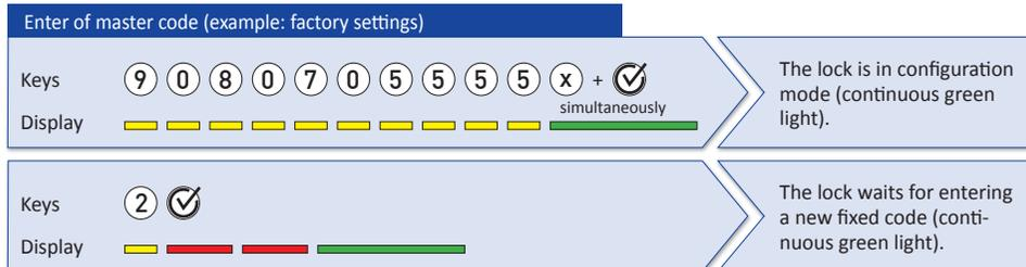
The LED display first flashes red twice after pressing the enter button and then turns to a continuous green light until a new fixed code has been entered.
