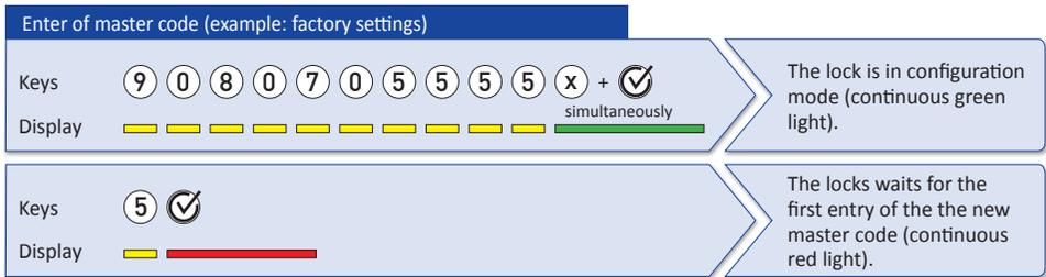
After the enter button is pressed the LED display will turn to a continuous red light until a new master code has been entered for the first time.
