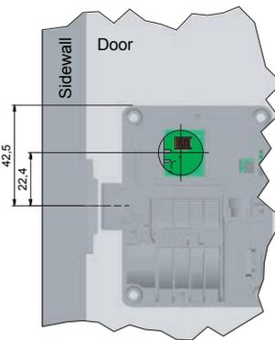
In order to attach the cover to the already mounted keypad unit TA03, insert the two guide lugs of the cover into the recesses and press the cover until it clicks into place.
