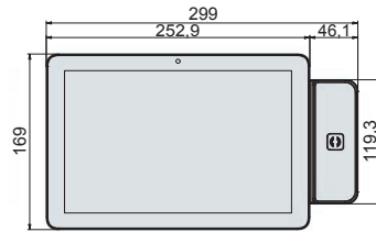
10" Central Control Panel with RFID reader Central Control Panel in 10" mit RFID-Leser
