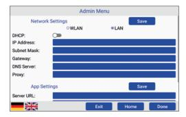
Alternatively, the Central Control Panel can be commissioned in online operating mode (LMS) by using the LEHMANN Data Transfer app on an NFC-enabled Android smartphone. To do this, hold the smartphone with the app in front of the RFID reader on the terminal. Enter the network settings in the app. Then hold the smartphone again in front of the RFID reader on the terminal.
