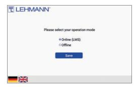
In the "Online (LMS)" operating mode, the terminal is connected to the LEHMANN management software LMS via LAN or WLAN. This operating mode is necessary for the "LMS Online Self Service" and "LMS Virtual Network" applications. Follow step 2 if you selected "Online (LMS)".
