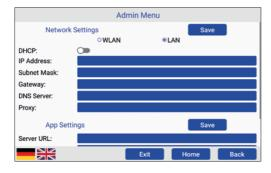
In the admin area of the online operating mode, the network settings for the Central Control Panel can be adjusted at any time. Enter the appropriate settings and click "Save". Then click "Back" to go to the application.
