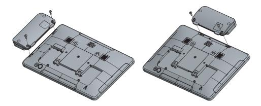
On the back of the terminal, remove the left cable cover by lifting it up.
