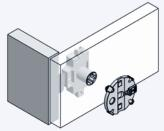
Attach P2|P4-adapter plate in open position
